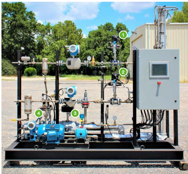
Figure 04: Multiple sliding gate valves by Schubert & Salzer are used in the Thermal Well Generator. (1) Fuel gas control valve (2) Air control valve (3) Well steam control (4) Vent steam control valve.
