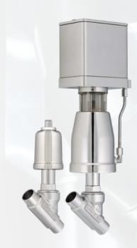
The hygienic angle seat valves type 7015 and 7025 have been designed without dead space. The batch numbers of all wetted stainless steel parts are traceable. The wetted plastics are FDA-compliant and conform to the EC Regulation 1935/2004 as well as the EU Plastic Regulation 10/2011.
